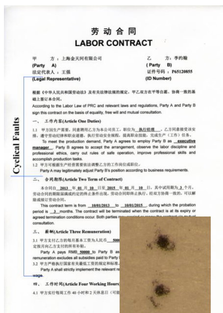
Fig.10 Cyclical defects on page 1
